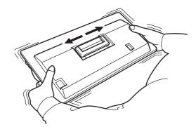
**7** Grasp the handle on the toner container and insert the toner container along the rail of the printer.
